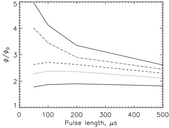
**Figure 3.** Ratio of the total magnetic flux generated by HF-pulses at 9 MHz and ERP = 95.7 dBW, X-mode for quiet nighttime ionospheric profiles, preheated by a long pulse at  $f = 4$  MHz, and ERP = 88.3 dBW, X-mode to that without preheating ( $\phi/\phi_0$ ) as a function of the short pulse length, for preheating by pulse lengths of 100, 200, 300, 500 s and by a very long pulse (from the bottom to the top respectively).
